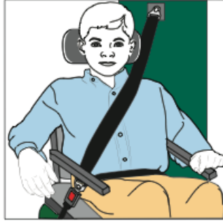
Good shoulder belt positioning over the center of the shoulder
