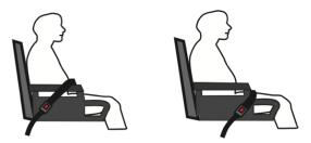
Improper positioning of the lap-belt portion of a vehicle seat belt over (left) and in front of (right) wheelchair arm supports
