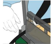
Lap belt placed in gaps between arm supports and the back support to achieve proper positioning low on the pelvis
