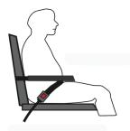
Proper positioning of a vehicle-anchored lap belt with wheelchair arm supports that are attached to the back-support posts and completely open at the front and underneath
