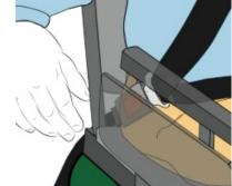
Lap belt threaded into opening between the wheelchair seat
