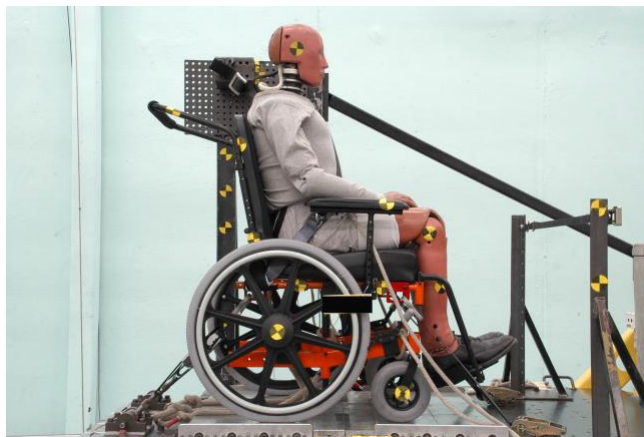
Figure 5 – Wheelchair secured facing forward on the UMTRI sled using the surrogate four-point, strap-type tiedown
