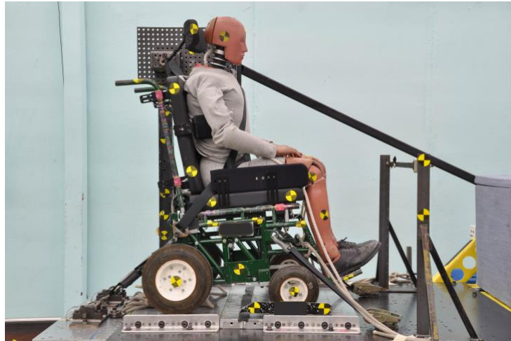
Figure 7 – Manufacturer’s seating system installed on the surrogate wheelchair frame (SWCF) secured facing forward on the UMTRI sled by the surrogate four-point, strap-type tiedown and loaded with a Hybrid-III midsize-male ATD
