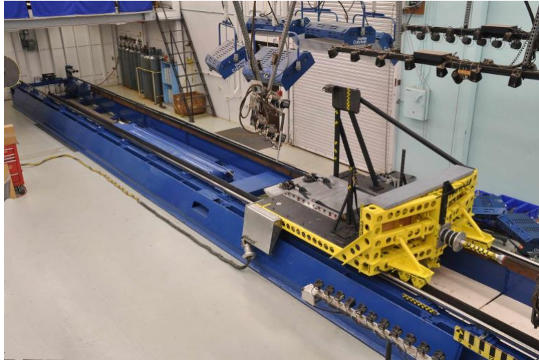
Figure 1 – UMTRI’s sled impact facility
