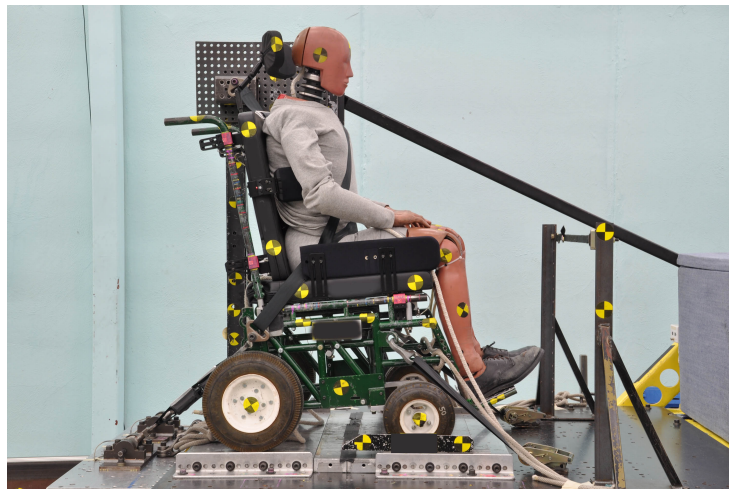
Figure 7 – Manufacturer's seating system installed on the surrogate wheelchairs frame (SWCF) secured facing forward on the UMTRI sled by the surrogate four-point, strap-type tiedown and loaded with a Hybrid-III midsize-male ATD
