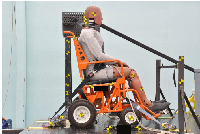
Figure 6 – 187-lb surrogate wheelchair (SWC) loaded with the Hybrid III midsize-male ATD restrained by a commercial lap/shoulder-belt restraint and secured facing forward on the UMTRI sled by the WTORS manufacturer's strap-type tiedown system
