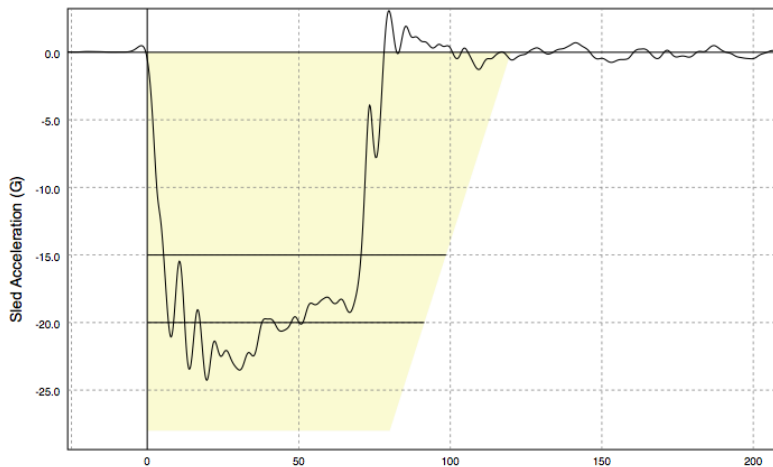
Figure 2 - Typical UMTRI 30-mph sled deceleration pulse compared to the corridor (shaded area) specified in RESNA and ISO frontal-impact test methods.
